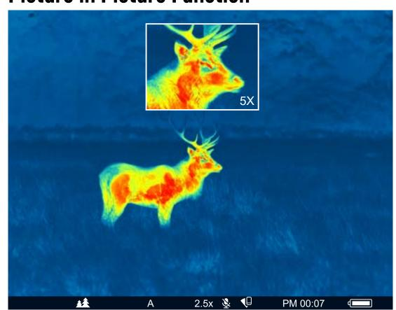
Picture-in-picture displays a magnified image at the top-center 10% of the overall field of view for precise zooming on an object of interest.
