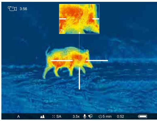
Picture-in-Picture improves accuracy by providing a magnified image of the reticle area at the top of the display. With only 1/10 of the display area reserved for PiP, the field of view remains virtually unobstructed for simultaneous PiP and FOV viewing.
